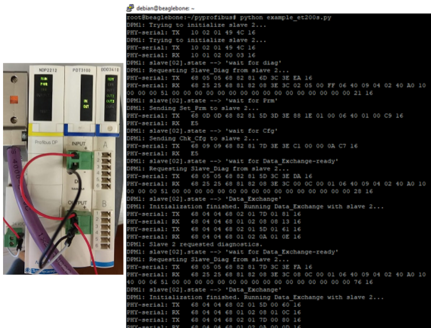
Figure 5.9: Example of a successful communication with a Profibus slave.
