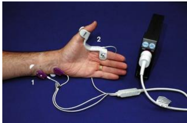
Figure 1.10 - Datex-Ohmeda M-NMT neuromuscular transmission module with kinemyographic mechanosensor. (1) Stimulating electrodes applied over ulnar nerve; (2) piezoelectric mechanosensor [39].
