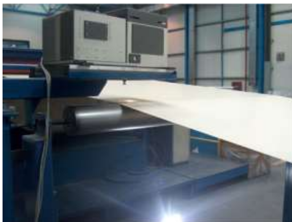
Figure 3.1.7. – Real time monitoring of paper' volatile content. Courtesy of Chimar Hellas S.A.
