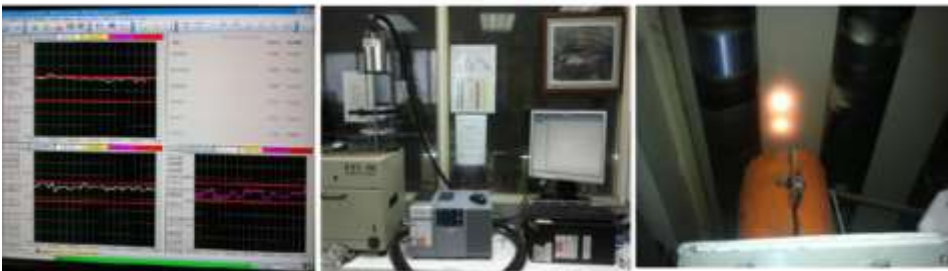
Figure 3.1.4 - a) On-line monitoring graphs of wood-based panel properties; b) Probe installed in a laboratory and c) On-line probe (Courtesy of Tafisa, Sonae Indústria (Valladolid plant)).
