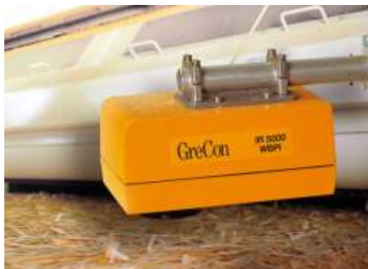
Figure 3.1.3 - In-line Moisture Measurement with Infrared Technology [45].
