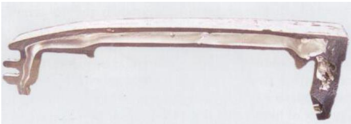
Figure 36- Zinc high pressure die casting with a cavity completely produced by gas injection [58].
