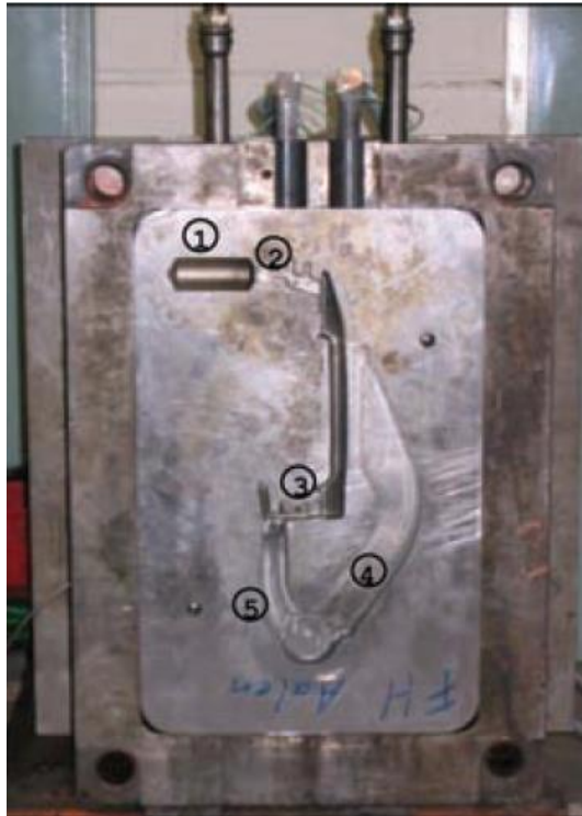
Figure 35- Pressure die casting tool for gas injection and a 200 ton cold chamber casting machine. 1- Overflow Cavity; 2- Locking Pin; 3-Injector; 4- runner; 5-Runner 2 [57].
