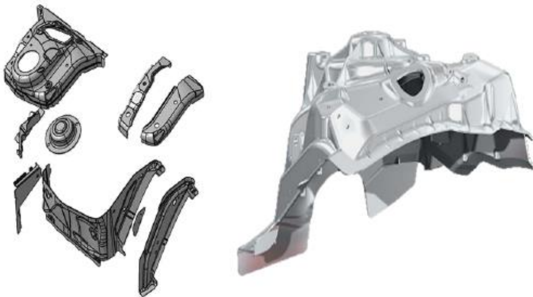
Figure 7- Left: Shock tower with an assembly of various sheet steel parts; Right: Same part with just a single part produced by aluminium die casting [10].
