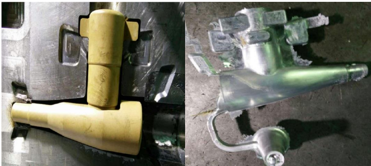
Figure 22- Left- “Triplet” salt core inserted in the die cavity; Right- Injected part of a zinc alloy [45].
