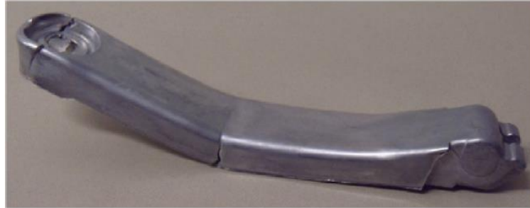
Figure 26- Deformation present on a manufactured part [52].
