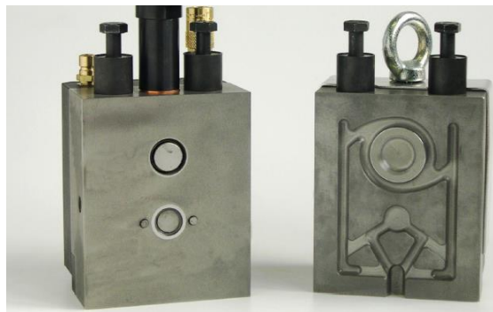
Figure 84- Mechanical shut-off vacuum valve with the Typhon vacuum runners [99].
