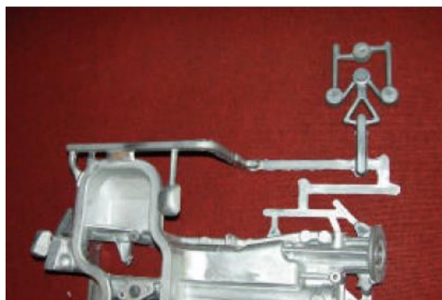
Figure 85- Vacuum runner for a mechanical vacuum valve [100].
