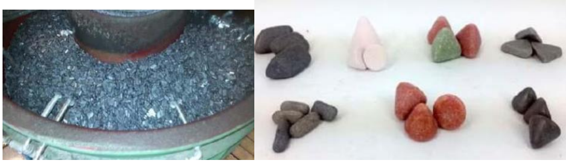
Figure 16- Left: Cast components being subjected to a grinding process; Right: abrasive chips [32].
