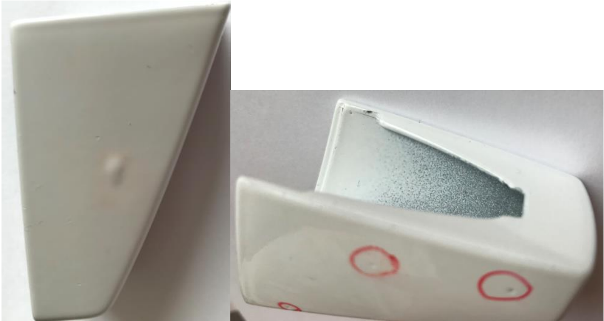
Figure 53- Left: Blistering; Right: Pin holes.
