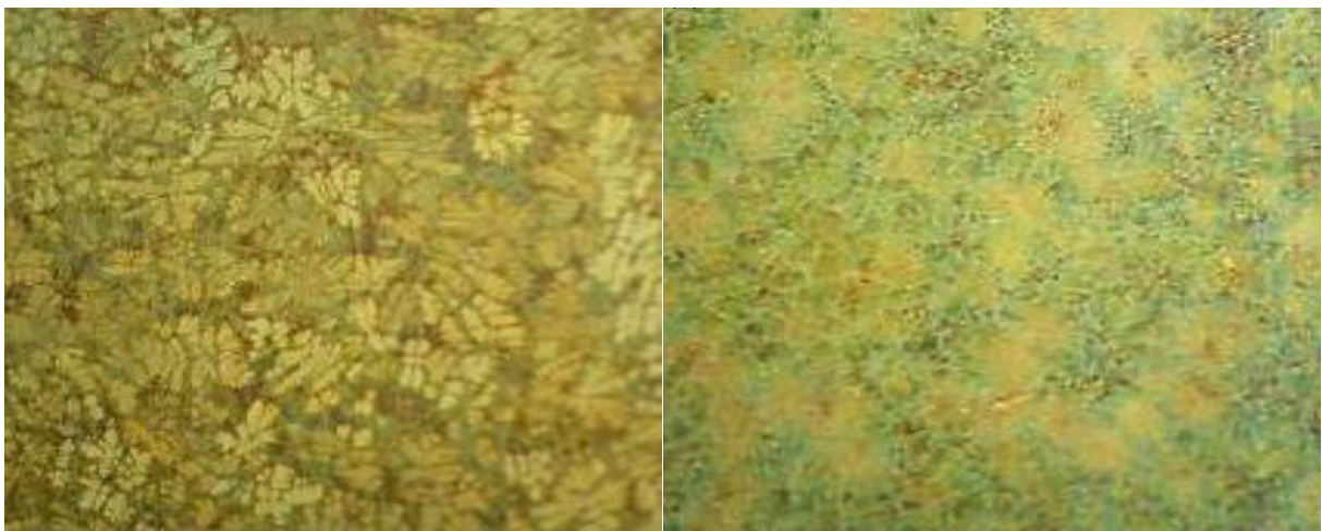
Figure 17- Left: Zamak 5; Right: Zamak 5 + 0.10 wt.% hf. Both allots at 200x magnification [35].
