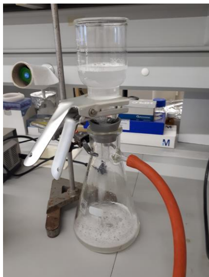
Figure D6 - Vacuum filtration system
