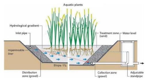
Figure 2.8 - Schematic representation of a constructed wetland. Adapted from Wang et al. (2017).
