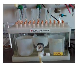
Figure 3.7 - SPE procedure.
