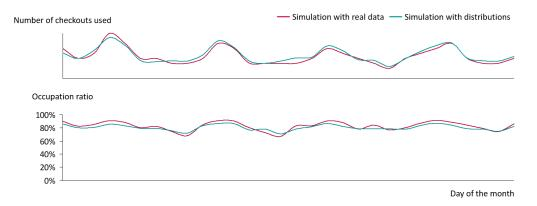
Figure 4.10: Comparison of the number of checkouts open and occupation ratio between the simulation model with real data and with distributions
