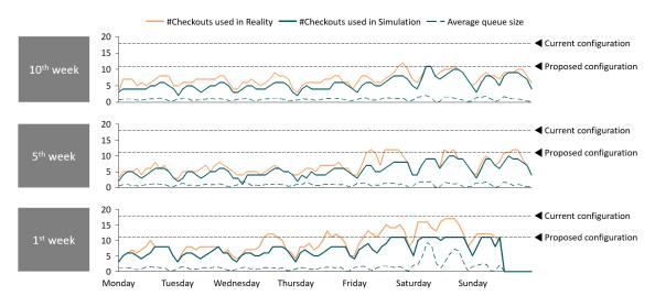
Figure 5.2: Number of checkouts used in reality vs in simulation and simulated average queue size. The average queue size could only be computed for the simulation scenario, since for the reality there is no record of the queue sizes' behavior in the represented weeks.
