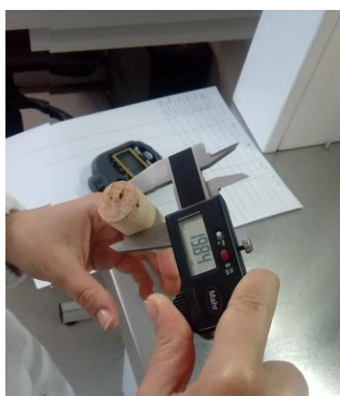
Figure 5 - Diameter measurements of the stoppers using a caliper, for the rebound recovery tests
