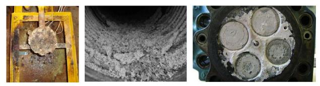
Figure 2 Acid corrosion, sulphur and silica deposits in engines after exposure to non-purified biogas (Arnold, 2009; BGS, 2018; EPA, 2002).
