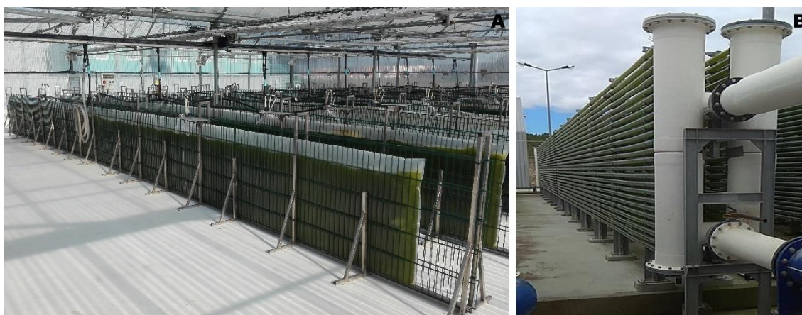
Figure 3.2. 1. Flat-panel reactor and tubular photobioreactor designs used for Nannochloropsis spp. scale-up: (A) 1000 L GWP reactors inside the greenhouse and (B) industrial scale PBR with 10500 L.
