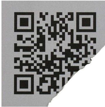
Figure7. Damaged QR code, is still decodable thanks to error correction. Image source: WikiPedia.
