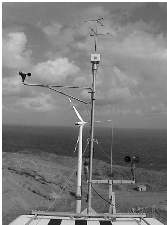
Figure 4.3: Experimental setup. The sonic anemometer METEK model USA-1 was mounted on the top of the main boom, and the NRG model 40 cup anemometer mounted below. The wind vane and anemometer from the wind turbine control system (not used in the experiment) can also be see in the bottom right of the picture.
