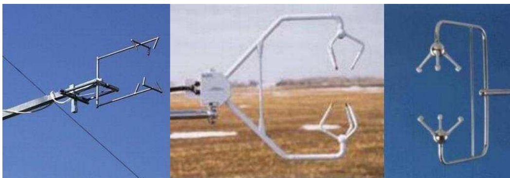
Figure 2.3: NUW, CSAT-3 and Gill HS sonic anemometers.
