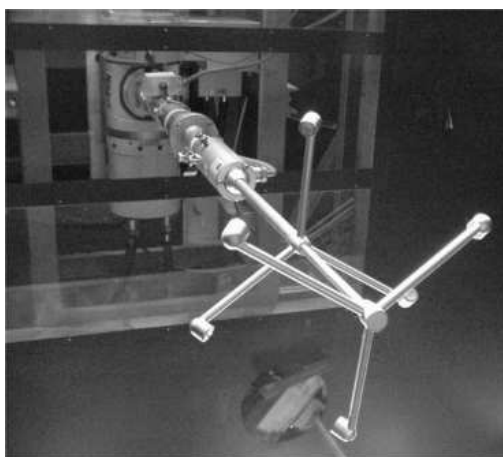
Figure 3.2: METEK (model USA-1) sonic anemometer coupled to the CNC-NIKKEN milling head.
