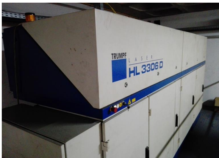
Figura 49 – Fonte laser HL 3306D (Trumpf) na Quantal S.A.
