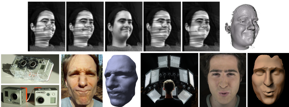
Figure 2.6: Examples of structured lights [ZSCS04] (top), stereo pair [VWB + 12] (bottom left) and 14-camera array [BHPS10] (bottom right).
