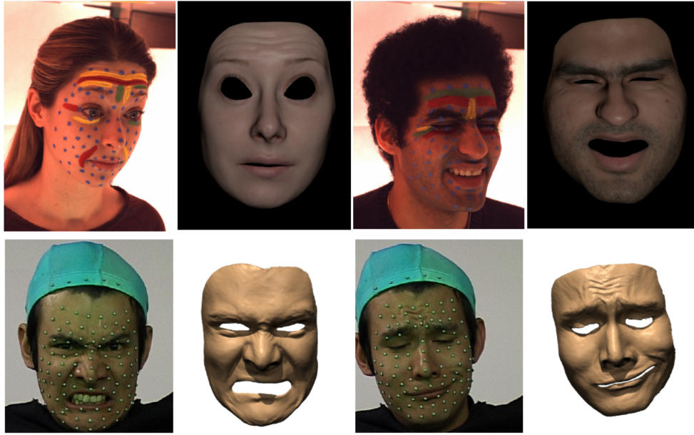
Figure 2.7: Examples of painted markers [BBA + 07] (top) and a marker-based (Vicon) set-up [HCTW11] (bottom).
