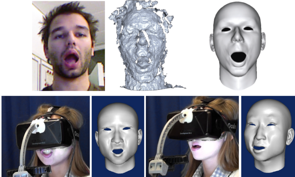
Figure 2.5: Examples of results obtained from RGB-D cameras. The top shows results from [WBLP11], while the bottom shows the results of [LTO + 15]. The latter additionally combines a thin membrane on the VR headset that measures the surface strain signals.
