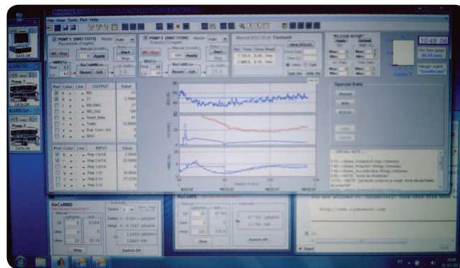
FIGURE 14 A computer display showing the GALENO anesthesia control system in operation, during one of the first tests in an early version of the platform. The display shows information concerning the control of neuromuscular blockade and depth of anesthesia, including the settings of the algorithm being used. In addition to tracking the reference, the associated operator interface allows changing between automatic (closed-loop) and manual control to administer to the patient a bolus of specified quantities of the relaxant or hypnotic drugs. The interface also allows including remarks—such as when the anesthetist manually administers a bolus of analgesic or when the electric bistoury is in operation—in the signal plots, which are useful for future interpretation of the data.
