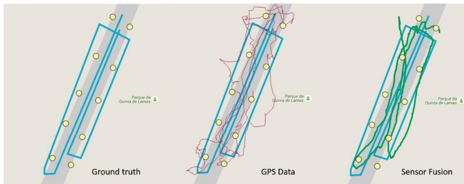
Fig. 5. Planned and estimated robot trajectory
