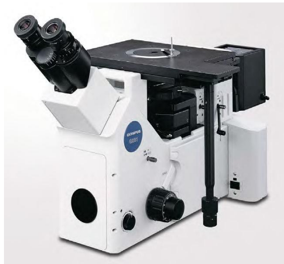
Figure 3.15: Metallurgical microscope used to observe the grain boundaries of the specimens
