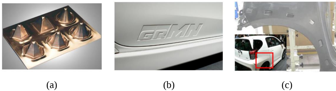
Figure 2.37: Application developed by Amino: a) Variety of pyramid shapes, b) Logo mark on Door panel of TOYOTA iQ-GRMN, c) Mounting boss on side panel of TOYOTA iQ-GRMN [84]
