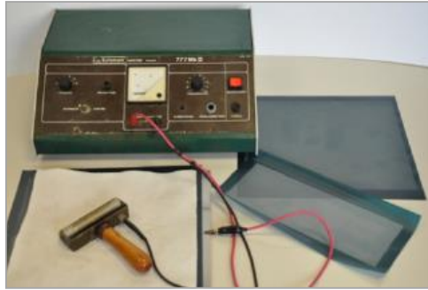
Figure 3.7: Electrochemical etching setup
