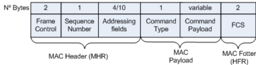
Figure A.6 – IEEE 802.15.4 command frame format
