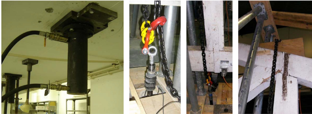
Figure 9. Details of the testing set-up: hydraulic jack and chain system for load application
