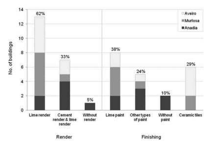
Figure 4. Coating of the outer surface of facade walls.
