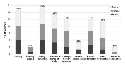
Figure 5. Common defects observed in facade walls.
