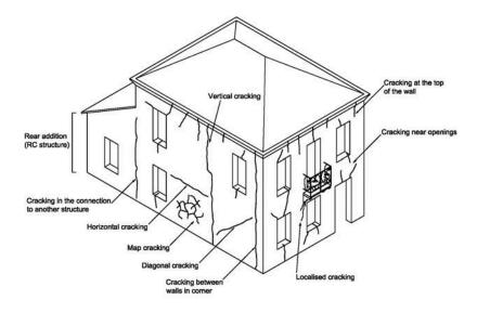
Figure 6. Schematic representation of the types of cracking observed in facade walls.
