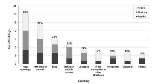
Figure 7. Types of cracking observed in facade walls.
