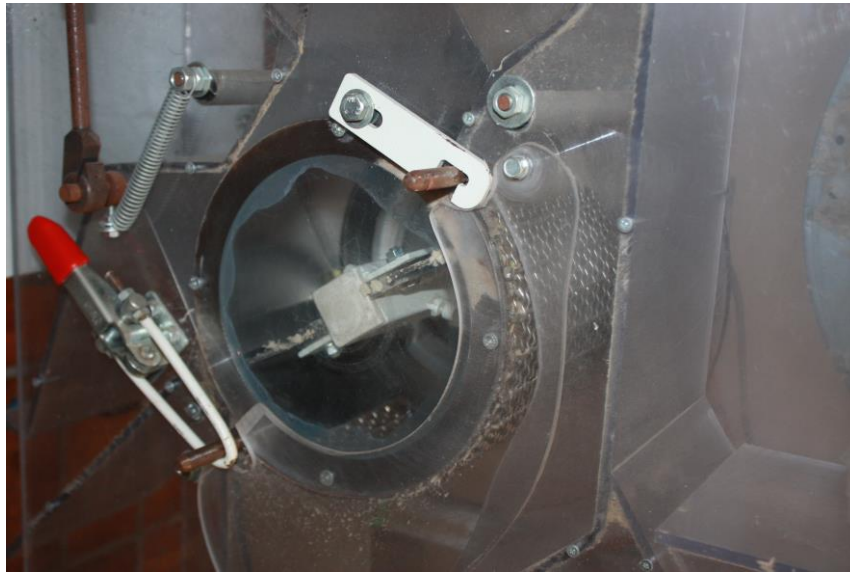
Fig. 44 – Threshing machine used after drying of the ears. Allowed separation of the kernels and hulls.
