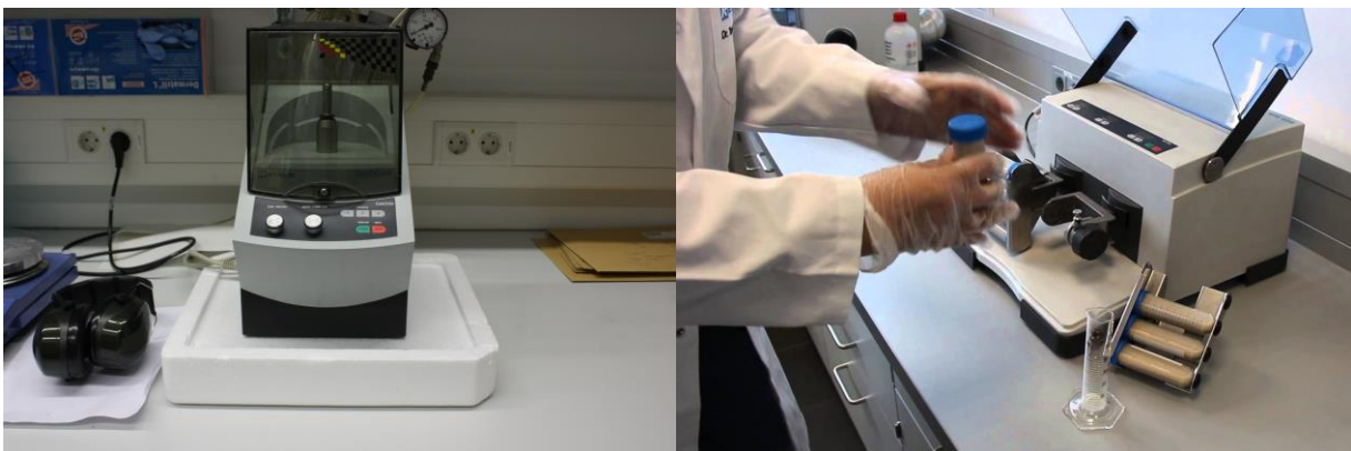
Fig. 46 – Retsch Grindomix GM200 (left) to mill higher amounts of plant material (10 ears, 10 leaves or 10 F-1 leaves) and Retsch MM400 (right) to mill smaller amounts of plant material, typically kernels and hulls that fit properly in the respectively two containers of the machine.
