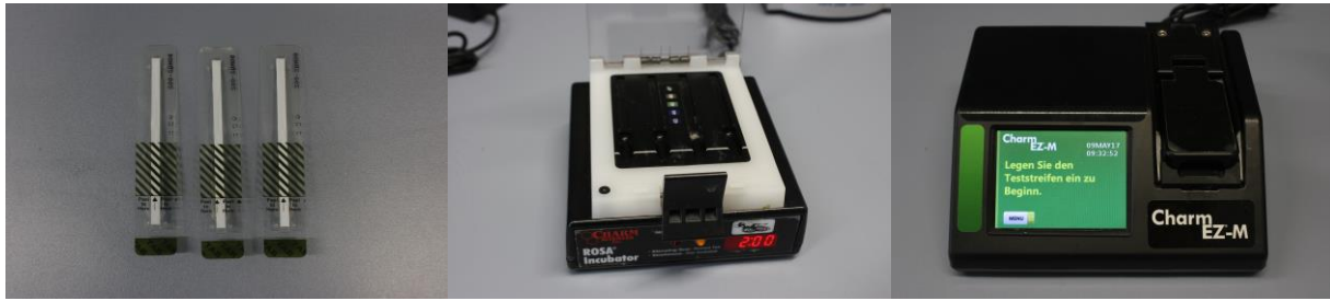
Fig. 47 – Prepared strips with 300 µl of sample (left). ROSA incubator (center) to put the strips for 2 minutes at 46°C and Charm EZ-M system to read DON concentration in the strips.
