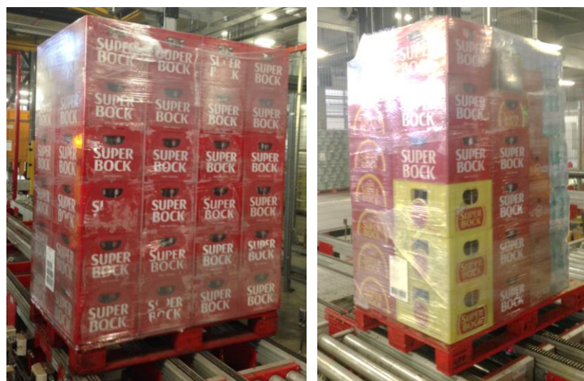
Figure 30 - Examples of pallets non-detected by the sensor
