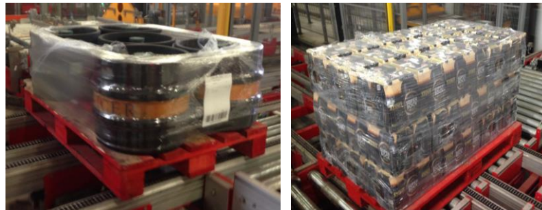
Figure 29 - Examples of pallets mistakenly considered as "Non-Good Bases for Stacking"
