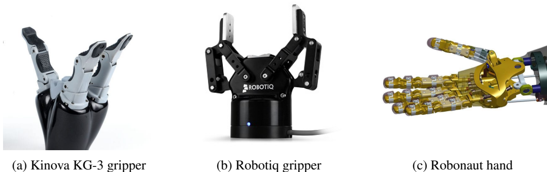
Figure 2.5: Examples of grippers for different applications: consumer (a), industrial (b) and research (c).
