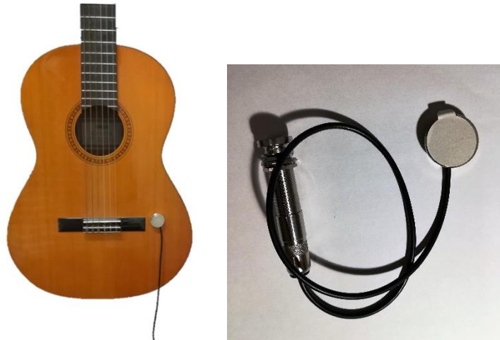
Figure 7.10 – Piezo electric pickup on the right, and piezo pickup installed on a classical guitar on the left.
