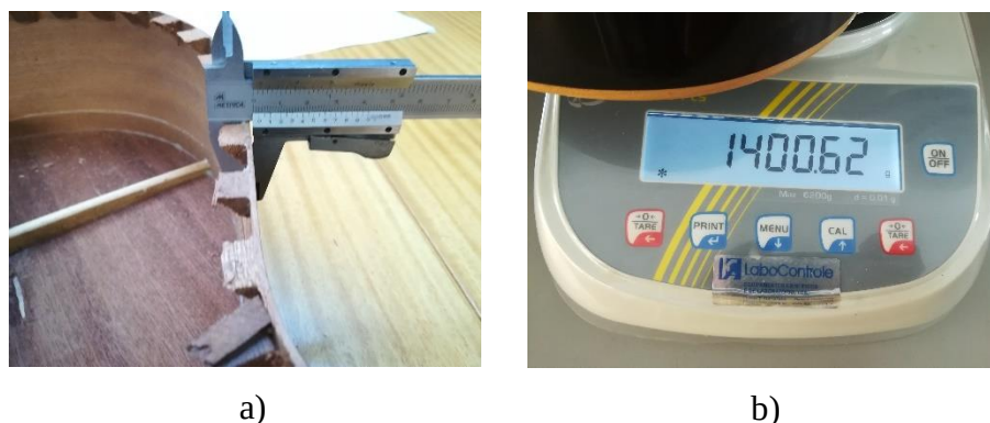
Figure 3.16 – a) Wall thickness measurement; b) Guitar weighting
