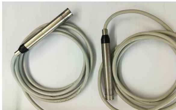
Figure 4.17 – Bruel &amp; Kjaer microphones type 4190, type 4165 right and left respectively
