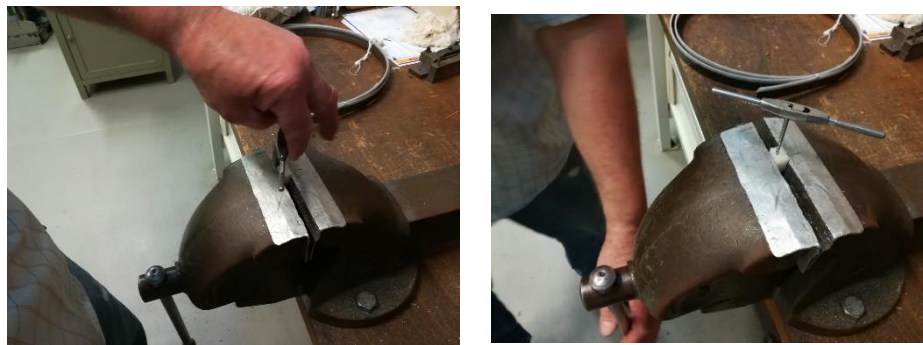
Figure 4.7 - Manual opening of a M2.5 screw thread
