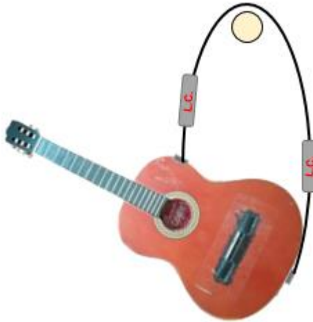
Figure 7.5 – Suspended guitar with load cells schematic
