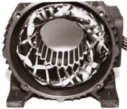
Figure 2.6: Typical induction motor stator [4].
