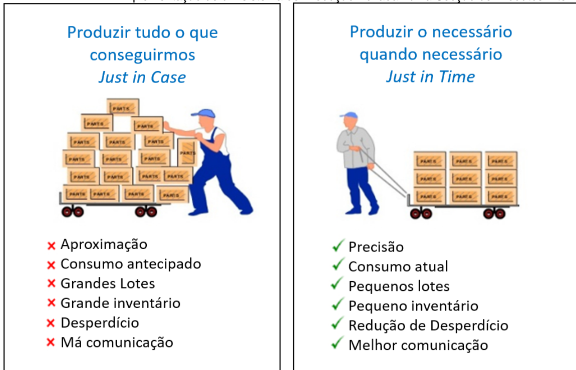
Figura 5 – Push vs. Pull (adaptado de: http://www.speedboard.co.uk/blog/6-benefits-kanban-system/ )
