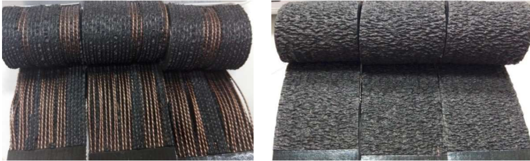
Figure 9 - Bad rubber-to-cord adhesion (left) Good rubber-to-cord adhesion (right).
