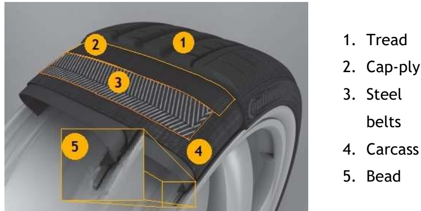
Figure 2 - Tire components (adapted from Continental, 2010).
