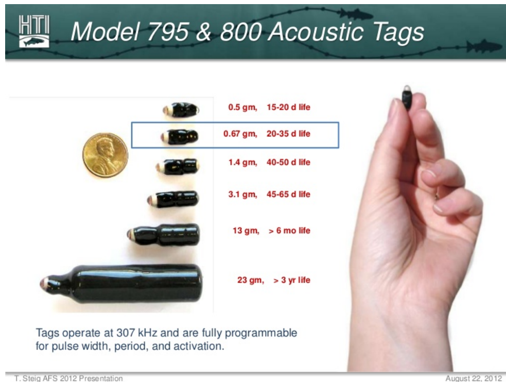
Figure 2.5: Size, weight and life period of acoustic tags
