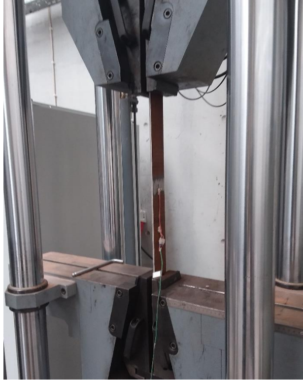
Figure 3.24 - Strip mounted in the Servosis MUF 404/100 universal testing machine
