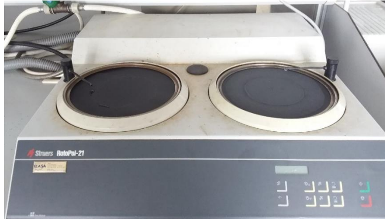
Figure 3.7 - Struers RotoPol-21 equipped with 320 and 800 grit SiC abrasive papers and tap water lubrication
