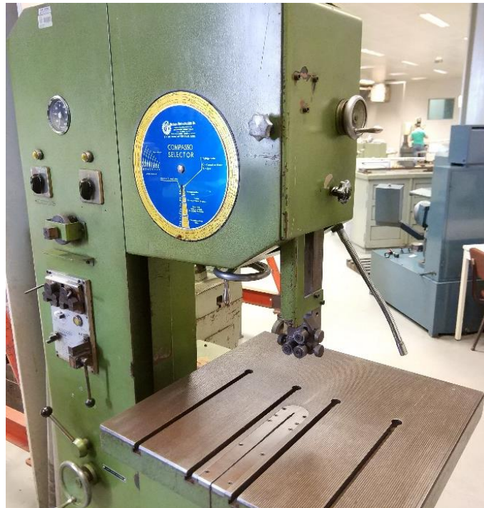
Figure 3.33 - Band saw used for the extraction of the specimens
