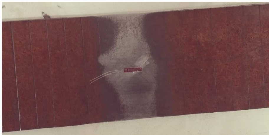
Figure 3.19 - Strain gage installed on steel strip
