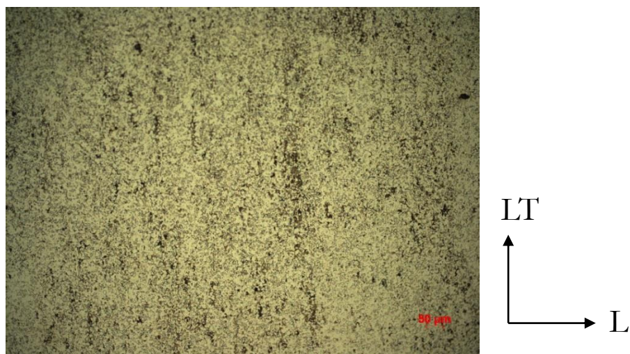
Figure 3.11 - Microstructure for the P355NL1 steel in the L-LT direction
