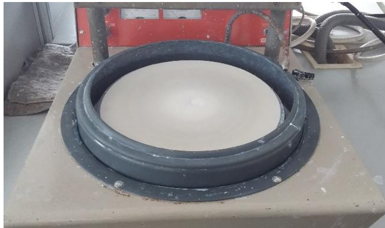
Figure 3.8 - Struers DP-U4 with felt disc and alumina suspension
