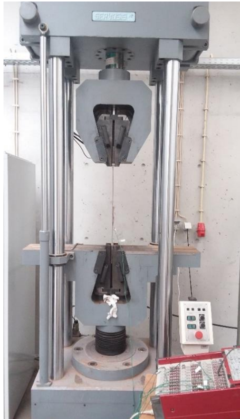
Figure 3.22 - Servosis MUF 404/100 testing machine
