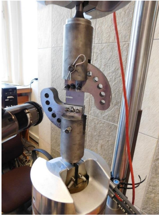
Figure 3.43 - CTS specimen during precracking procedure (pure mode I)
