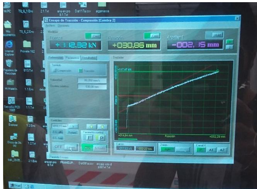
Figure 3.25 - Test screen with load-position plot and instant values of displacement and force
