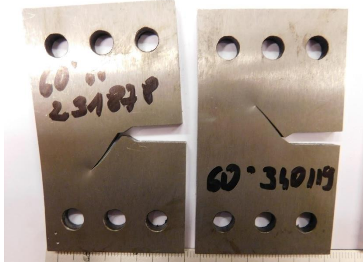
Figure 4.20 - Pre-strained (left) and non-prestrained (right) specimens after the crack growth test ( \alpha=60^\circ , R=0.5 ).
