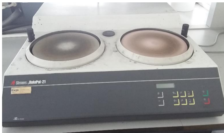
Figure 3.9 - Struers RotoPol-21 with diamond spray
