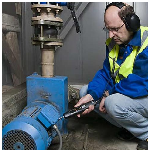
Figure 2.4 - Audible monitoring with an electronic stethoscope [8]
