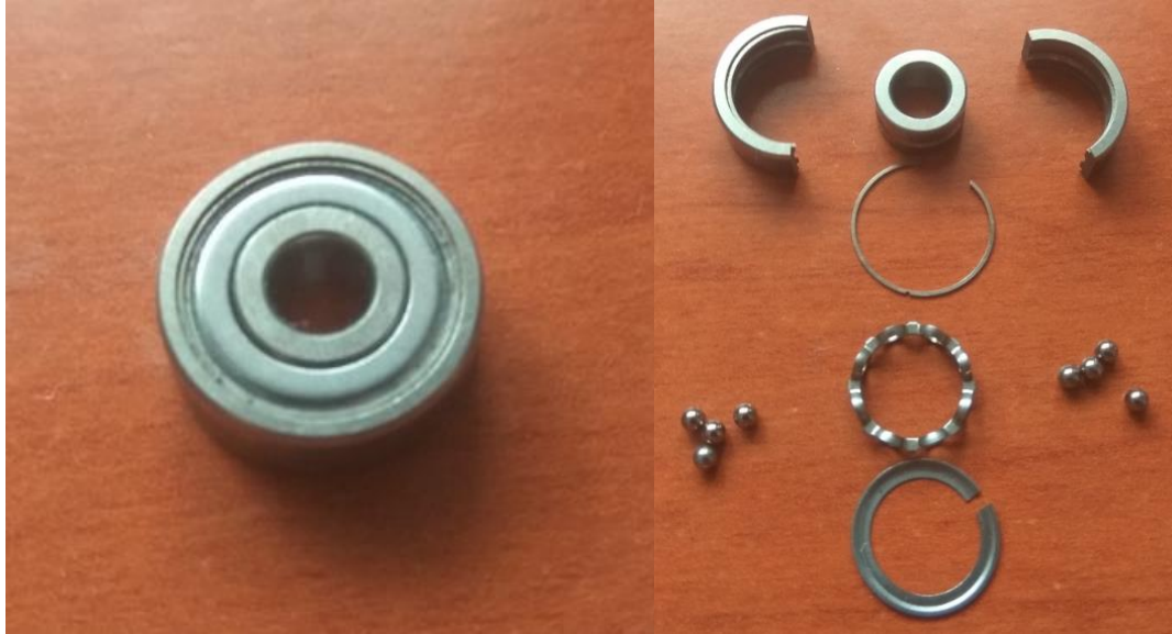
Figure 4.2 - Anemometer's bearing; mounted (left) and cut (right)
