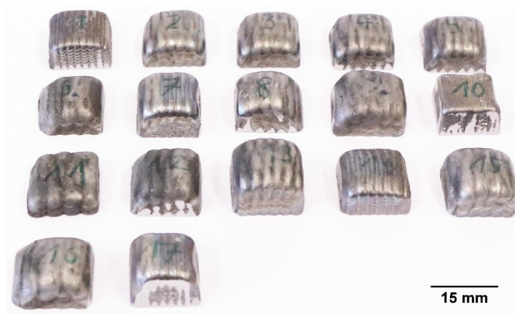
Figure 32 - Inconel 718 cubes made by DED process on TruLaser Cell 7020.
