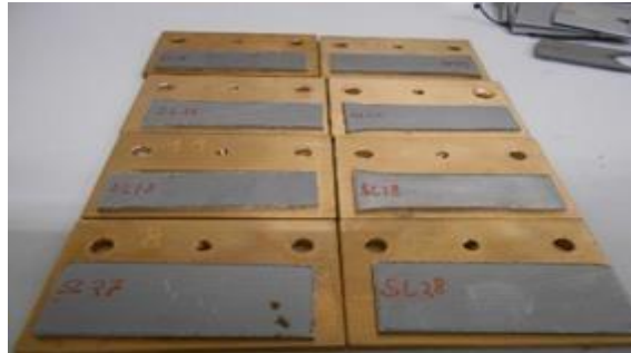
Figure 3.2 Test samples of the steel sheet are stacked on the plate
