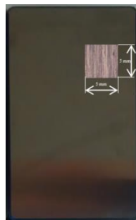
Figure 4.10. Measured surface area 5x5 mm 2 , tool surface Grinded along the Sliding direction
