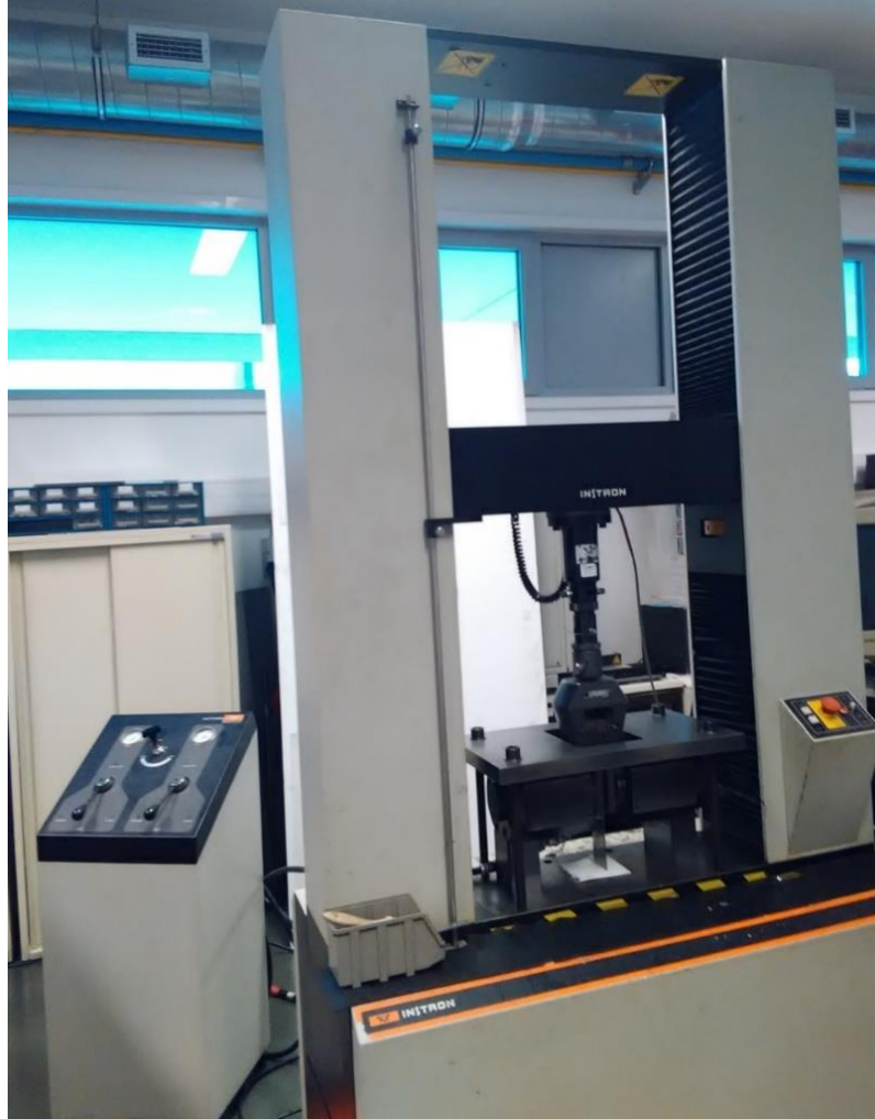
Figure 4.2 Tensile testing machine and modified strip drawing tribotester
