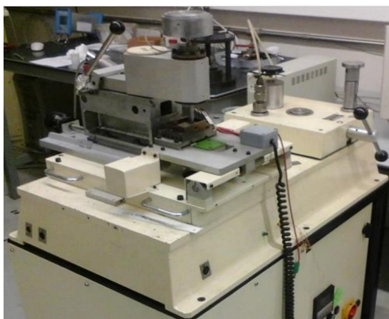
a) General view of the reciprocating attachment
