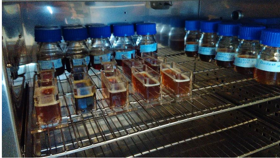
Figure 3.3 Preparation of combined lubricants for viscosity measurement
