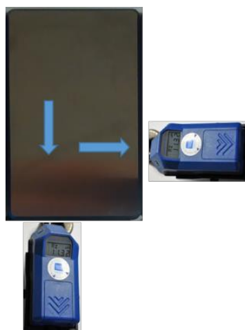
Figure 4.13 Method of measurement of tool surface with traditional HOMMEL TESTER T500
