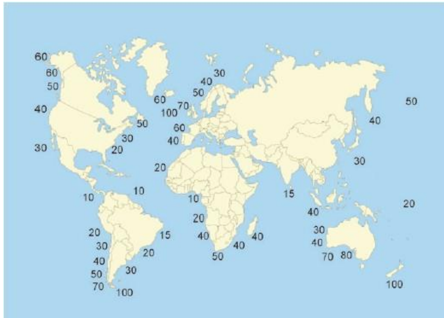
Figure 7- World wave energy resource. The numbers represent average energy flux [kW/m] (Waters 2008)
