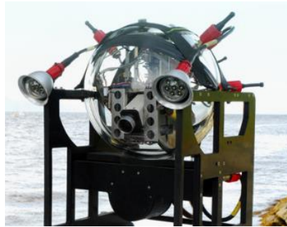
Fig. 4 Hybrid Remotely Operated Vehicle 11k from Promare
