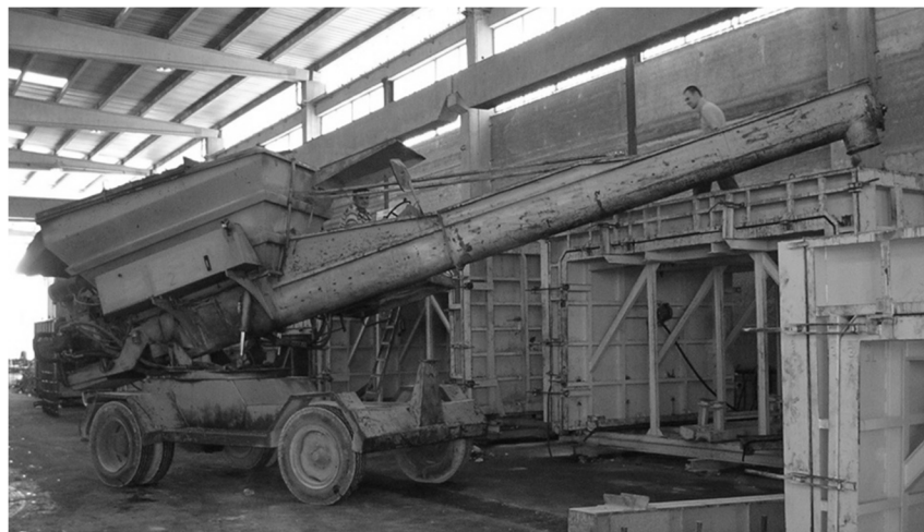
Figure 2.1 – Motor-vehicle used to transport and cast concrete.
