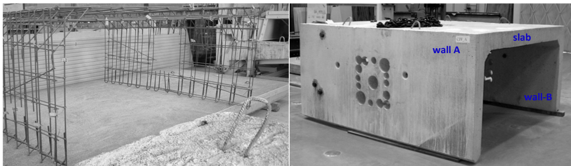
Figure 2.4 – Box-culvert element: reinforcement and location of test cores in side-wall A.
