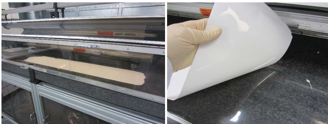
Figure 30: Aspect of the ceramic tape after casting and flexibility in the green state
