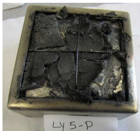
Figure 25: (a) Heat release rate curves of 5 wt% FR filled epoxy resin (b) residue of 5% ATH filled resin (c) residue of 5% APP filled resin
