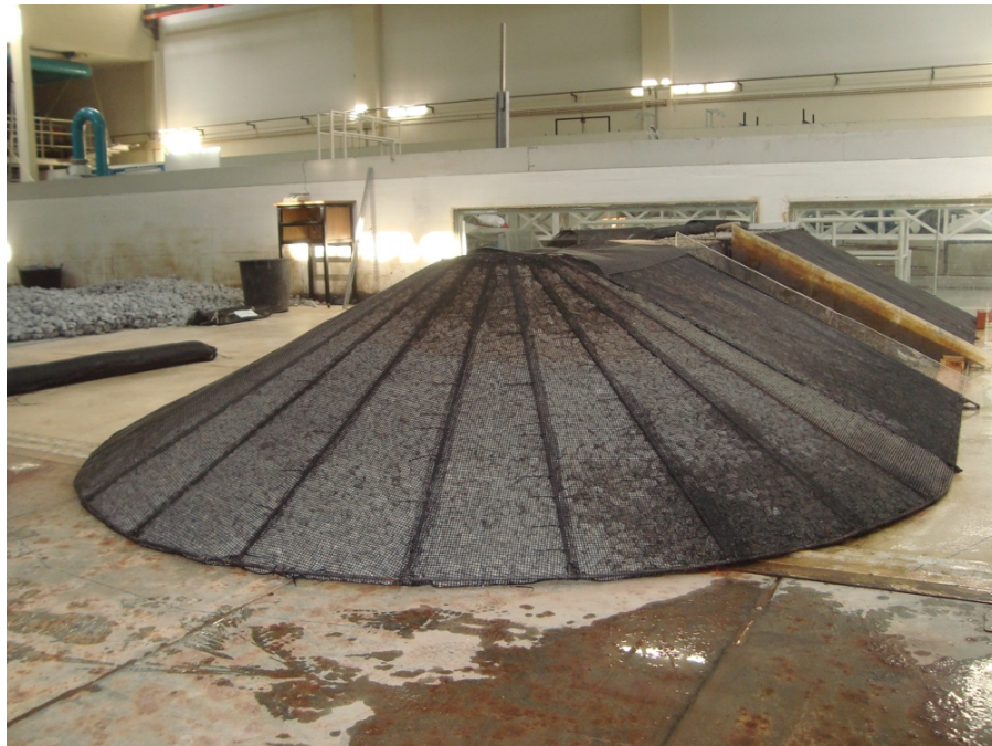
Figure 3.18 - Physical model of a rubble-mound breakwater, inside the wave tank of the Faculty of Engineering of the University of Porto (FEUP, 2016).
