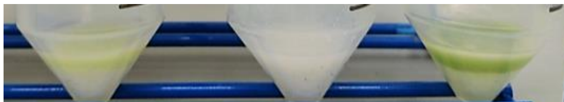
Figure 8. Appearance of the Q2 wastes after the clean-up step with each one of the extracts performed with the different solvents tested, (from left to right, Hex/DCM, n -hexane and Hex/Acet).
