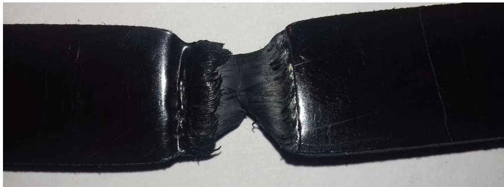
Figure 80 – Deformation on the parent material in specimen 3 of the confirmation test.
