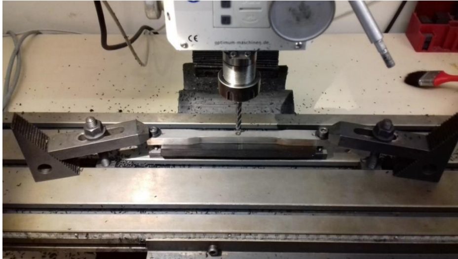
Figure 34 – Machining of HMWPE 3mm sheets into normalized specimen.
