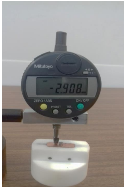
Figure 46 – Probe length measuring with a micrometer.
