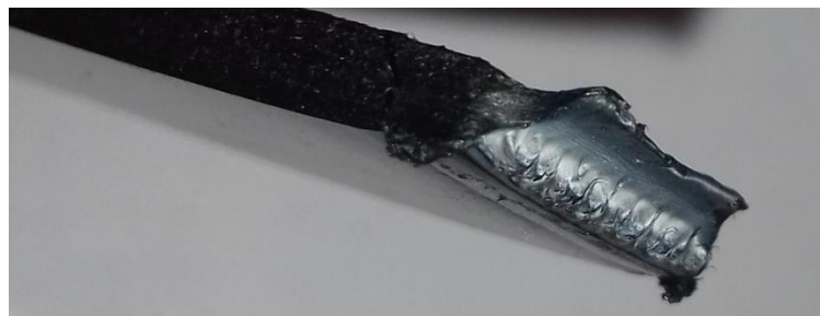
Figure 76 – Semi-brittle fracture of the specimen 2 of the test S(5,1).
