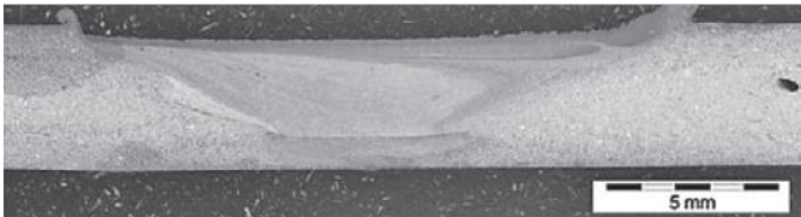
Figure 28 – Weld flash due to excessive heat input [40].
