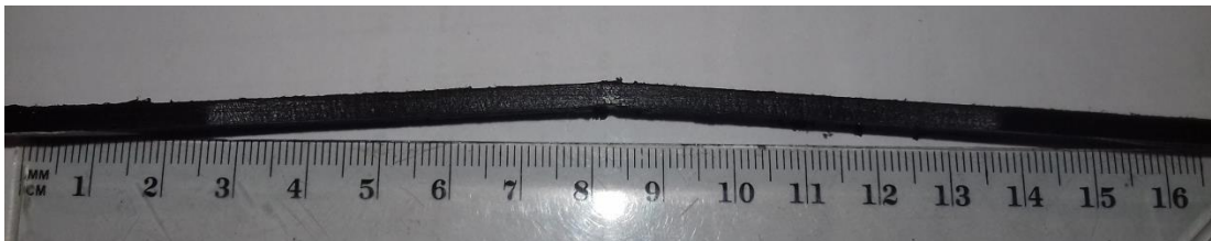
Figure 72 – Example of flexural deformation caused by the welding process forces, test S(9,2).
