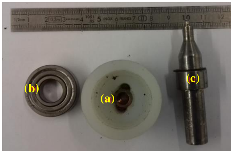
Figure 38 – Pre-test stationary shoulder tool: a) shoulder; b) bearing; c) tool body with 3mm probe.
