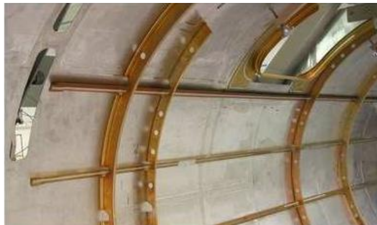
Figure 19 – Skin, stringers and frames joined via friction stir welding in eclipse jet [33].
