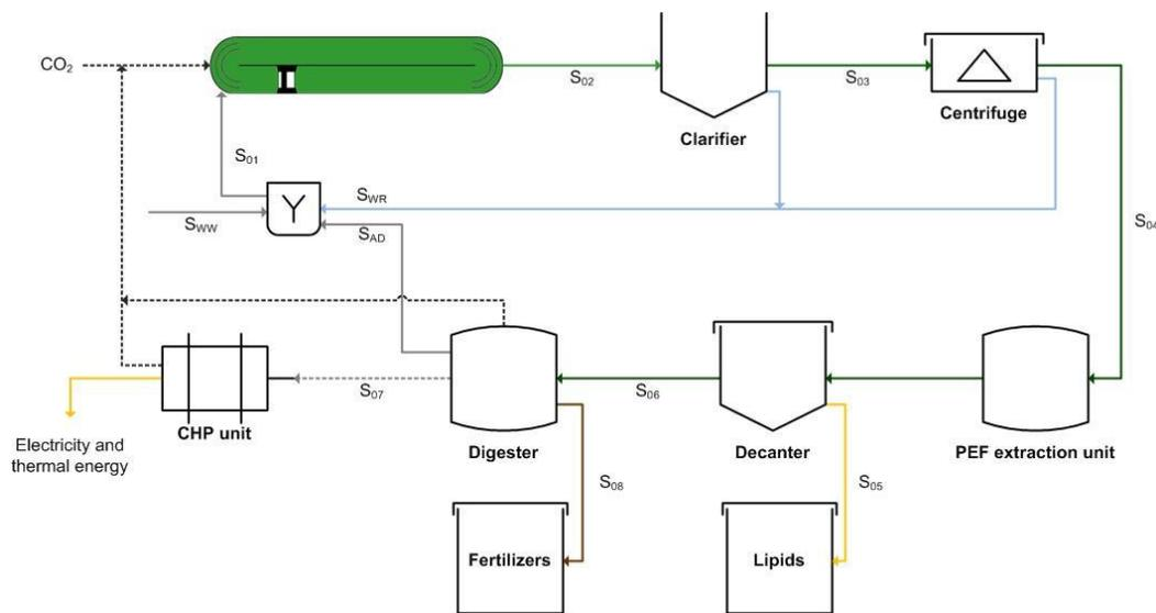
**Figure 2.** Process diagram. CHP—combined heat and power; PEF—pulsed electric field.
