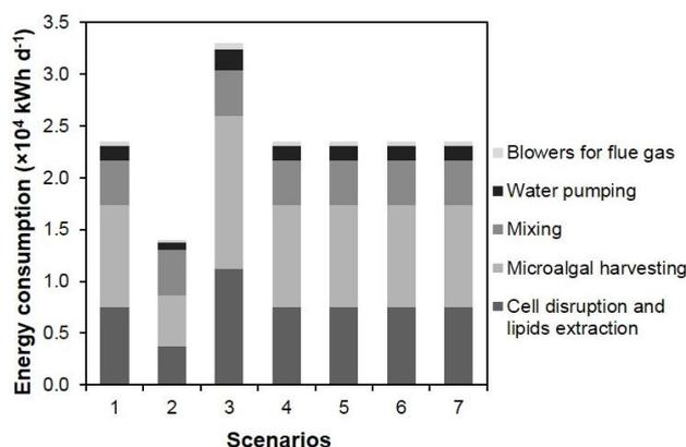
**Figure 3.** Electrical requirements determined for different steps of the microalgal facility in each of the studied scenarios.
