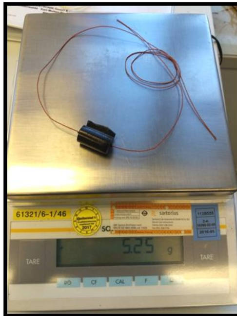
Figure 60 - To weigh the sample, make sure that the entire cord is on the plate
