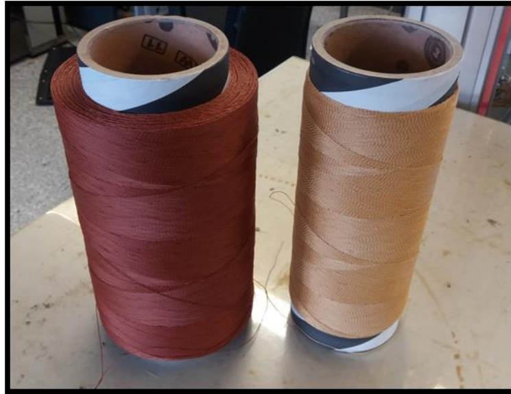
Figure 58 - Textile cord with RFL system (left) and without (right)
