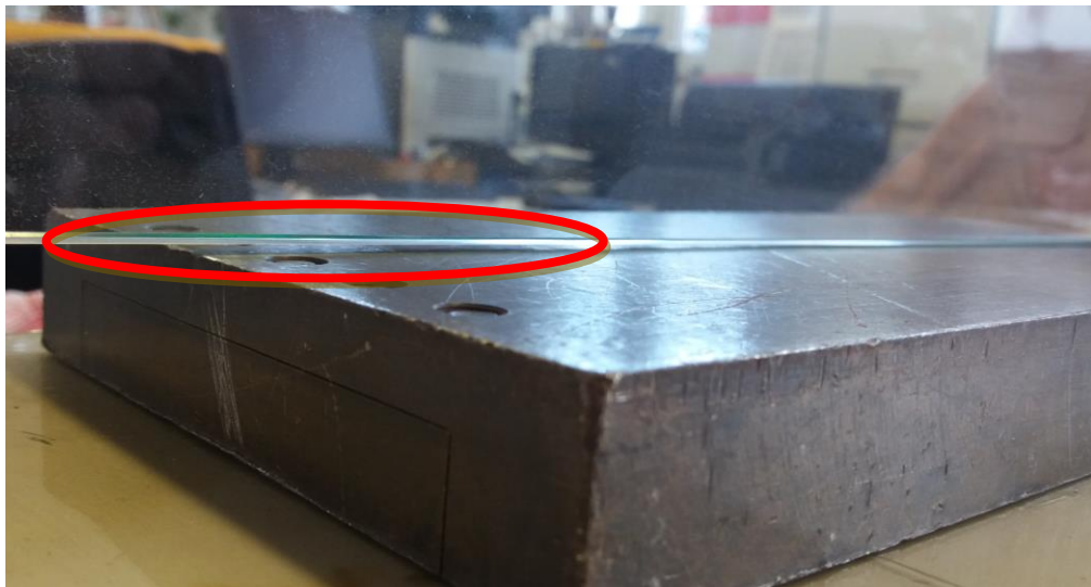
Figure 55 - Mold's gap detected using a glass surface.
