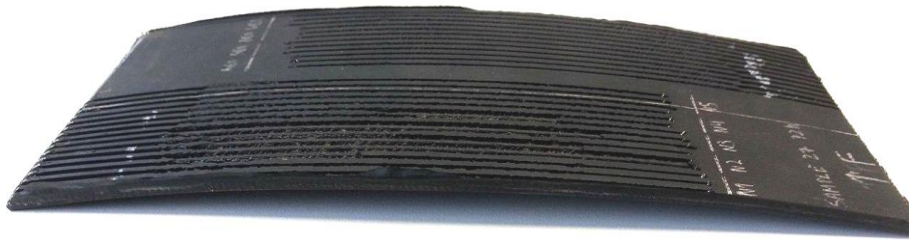
Figure 38 - Natural bending of the sample for a back layer with 90°
