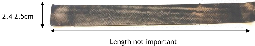
Figure 56 - The length of the stripe varies according to the rubber sheets provided
