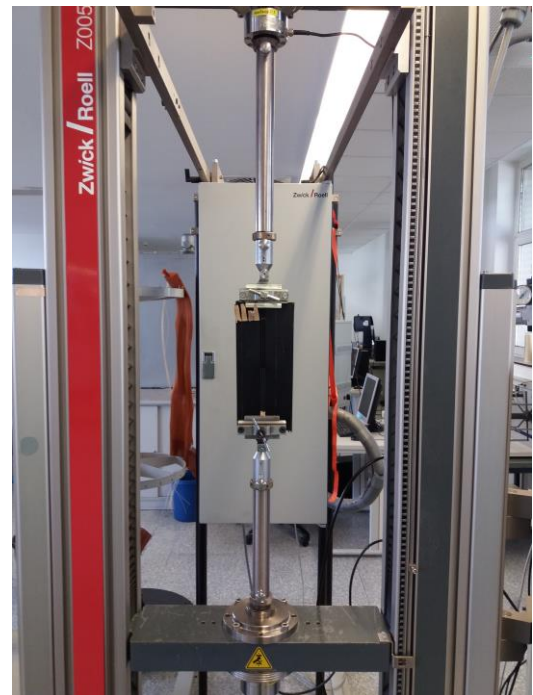
Figure 12 - 3 Cord Adhesion Test - Peeling of the steel cords
