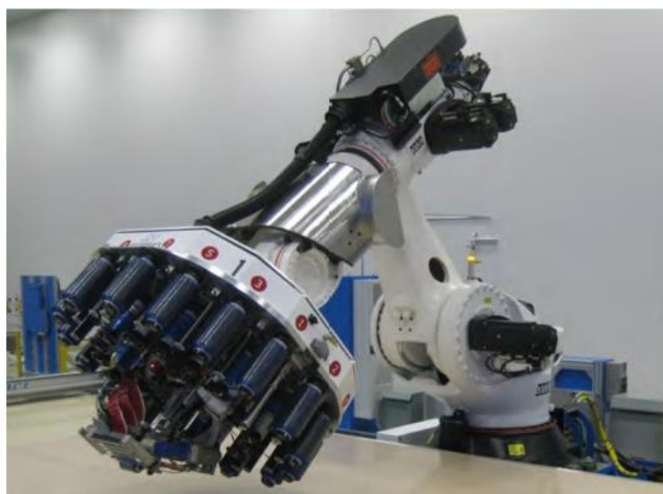
Figure 7 – AFP material delivery head(Jeffries, 2013)
