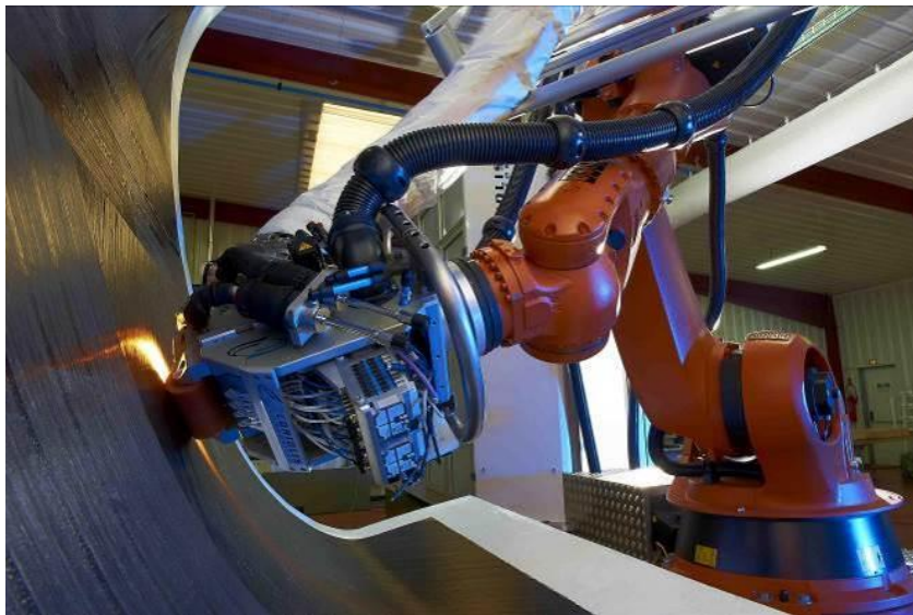
Figure 6 – ATL material delivery head ( http://www.mmsonline.com/news/coriolis-composites-enters-long-term-partnership-with-dutch-tprc )
