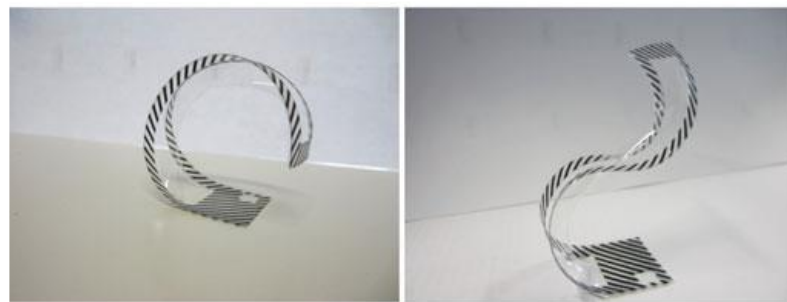
Figure 11 – States of dielectric elastomer minimum energy structures(Araromi et al., 2015)
