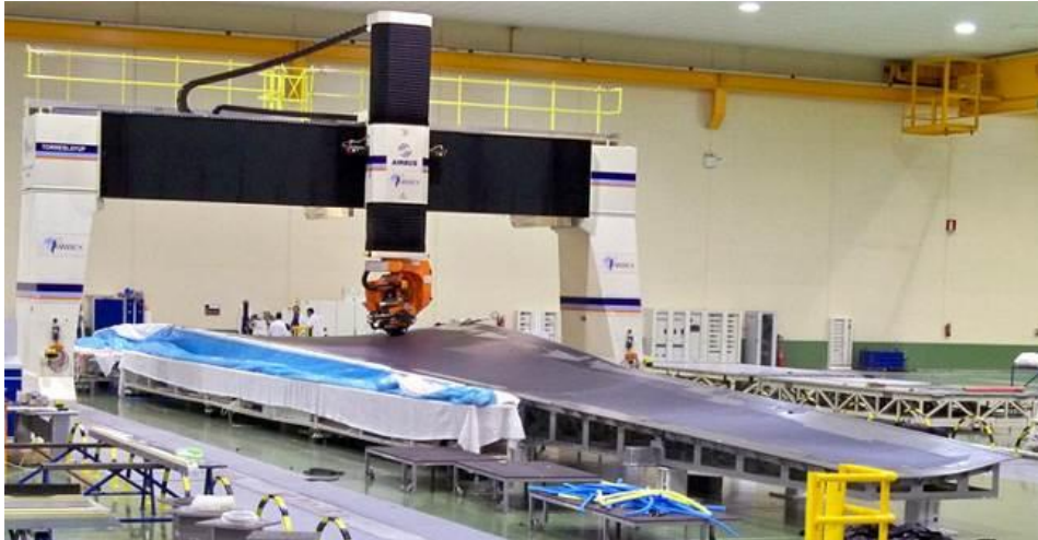
Figure 5 – ATL configuration ( http://australianaviation.com.au/2010/09/airbus-flight-tests-a350-composite-panel/ )
