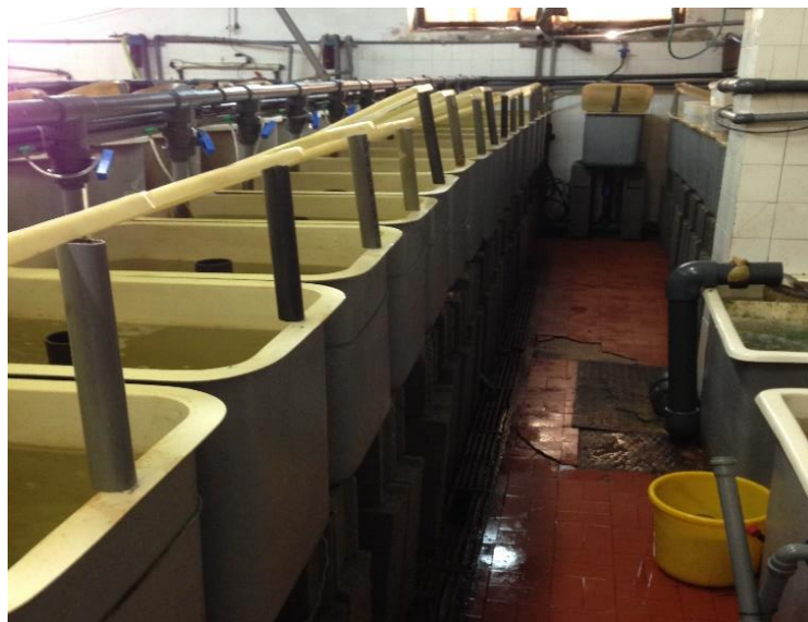
Fig. 5: Thermoregulated recirculation water system used for the growth trial.
