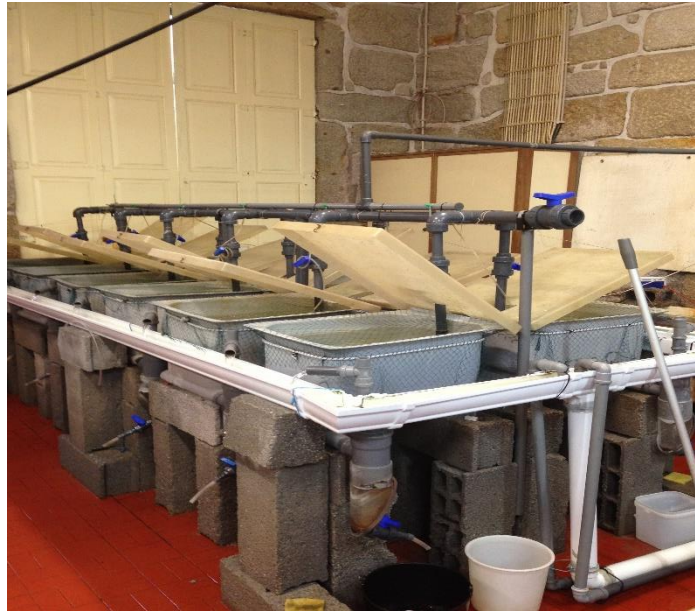
Fig.8: Thermoregulated recirculation water system used for the digestibility trial.
