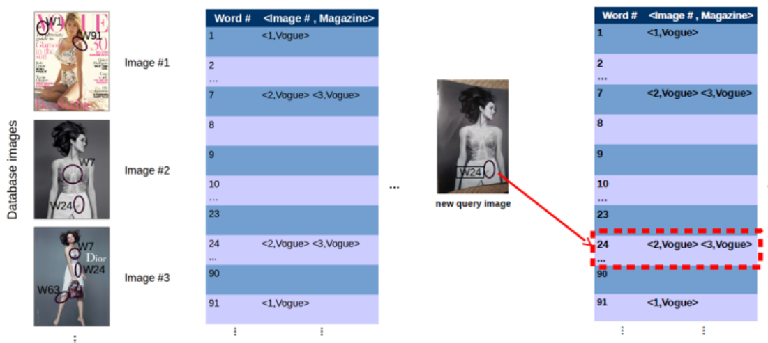
Figure 4.5: Illustrative example of the efficient indexing structure developed. Left: All database images are loaded into the index mapping visual words to image numbers. Right: A new query image is mapped to indices of database images that share a visual word.
